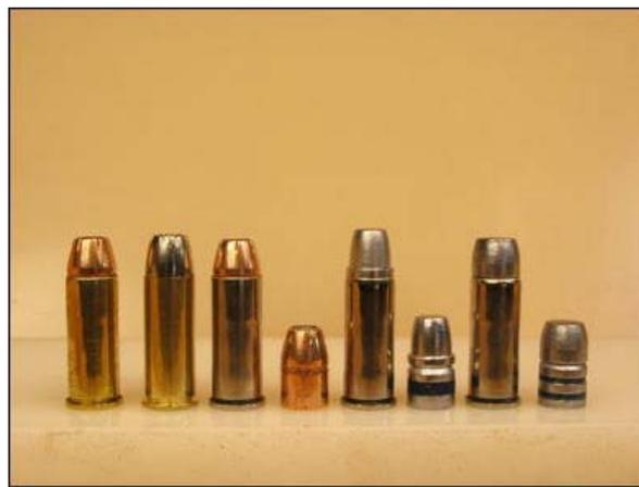
*Two factory loads and reloads from left: 180 gr Hornady XTP, 200 gr. Winchester Silver Tip, 240 grain Hornady XTP, 250 grain Keith, 280 grain LBT.*
