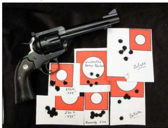
*The 5 1/2-inch revolver with some of its targets. The two on the right are before I cut the Taylor throat in the barrel. The rest are after, with a variety of jacketed and cast bullets.*
