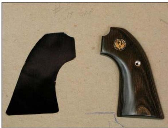
*The modern Ruger Bisley grip on the right is shown with a tracing I made of the Keith No. 5 frame. The Ruger Bisley is virtually identical to the wonderful custom revolver from the 1920s.*
