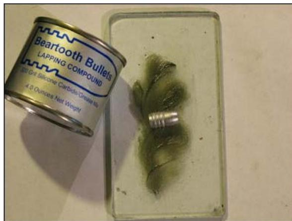
*Fire-lapping bullets are made by rolling bullets in special abrasive compound.*
