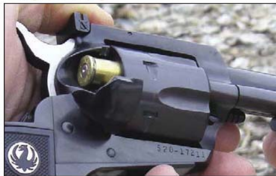
The Ejector Alignment Pawl aids in chamber alignment with the loading trough and was first employed in the 50th Anniversary Blackhawk .357. It also allows easier loading and unloading.
