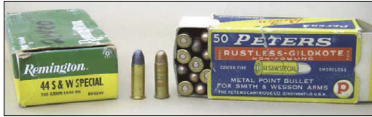
Left, the .44 Russian (left) was developed around 1870 and was a black-powder round. The .44 S&W Special (middle) was essentially a lengthened Russian case and was loaded with both black and smokeless powders in 1907/08. The .44 Remington Magnum (right) was developed in 1955 and was simply a lengthened .44 Special case and loaded to significantly greater pressures. Above, the .44 S&W Special has traditionally been loaded with a 246-grain roundnose bullet at an advertised 755 fps. Through handloading, performance can be improved.
