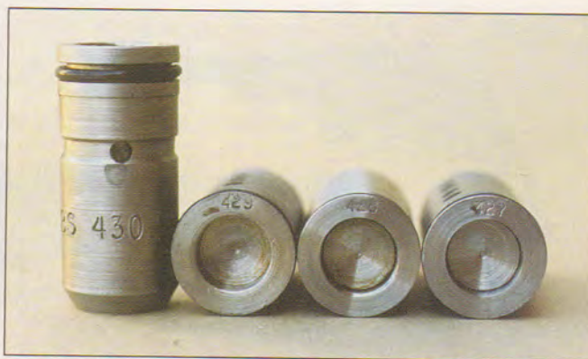
H&I sizing dies are available in .427, .428, .429 and .430 inch, allowing cast bullets to be sized accordingly.
