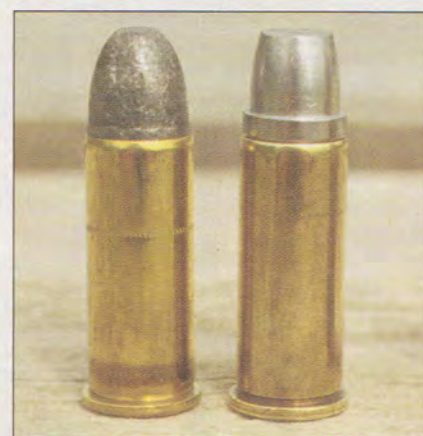
Above, the original 246-grain roundnose factory .44 Special load remains available, but some companies have increased velocity using lighter bullets. Buffalo Bore offers a 255-grain cast SWC at 1,000 fps for post-World War II guns only. Right, the original .44 Special 246-grain factory load (left) is advertised at about 755 fps. The handload contains a 250-grain Keith-style cast bullet loaded to 1,200 fps.
