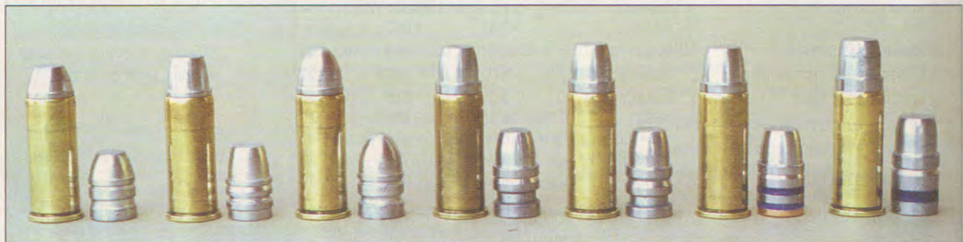
A variety of cast bullets was used in compiling load data. Left to right: RCBS 44-200-FN, Lyman 429215 220 grains, Lyman 429383 245 grains, Lyman 429421 250 grains, RCBS 44-250-K 255 grains, Lyman 429244 255 grains and Dry Creek SWC 307 grains.
