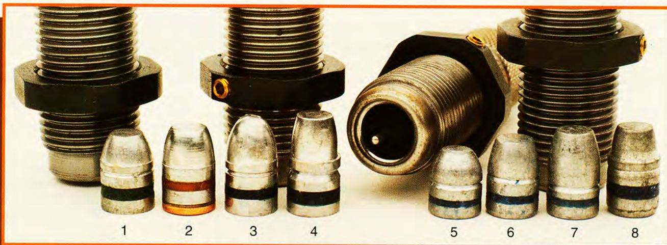
Current Lyman .44 Special dies include a fourth die for use with powder measures on progressive reloading machines. Representative cast bullet designs for the .44 Special include (1) RCBS 44-200, (2) Lyman 429434, (3) Lyman 429383 and (4) RCBS 44-250 Keith. Commercial bullets from Double A Limited (5, 6 and 7) range from 175 grains to 240 grains. The (8) Bull-X 240-grain semiwadcutter is cast from a relatively hard alloy that is intended for magnum pressures and velocities.
