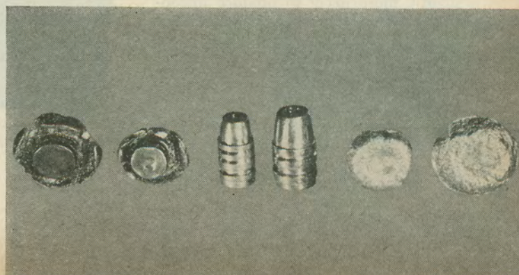
Greater expansion of .44 Special over Magnum bullets is shown here. Impact velocity approximates that at 100 yards. The .44's were moving at 1000 f.p.s.; the Magnums at 1300
