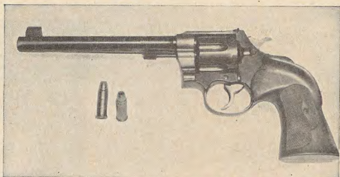
The .44 special magnum cartridges and Colt Officers Model they are used in, showing the custom grips Walter Roper designed to minimize recoil
